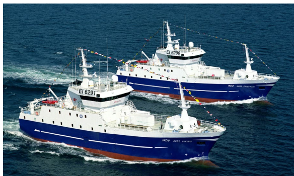
AVRO CHIEFTAIN & AVRO VIKING Yard UMOE Sterkoder AS. Gearbox G50F Propeller P70.23.260.4 – ICE C Engine 1 650 kW-1000rpm.
