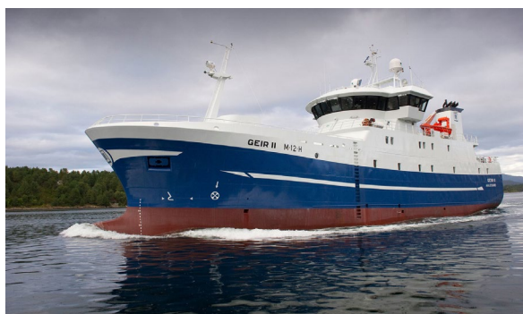
GEIR II Yard Fiskerstrand V. AS Gearbox G60F Propeller P70.24.270.4 – ICE C E-motor 1800 kW-1200rpm.
